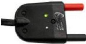
3. Connect the Security Test Device to the battery's charging connectors making sure the connector body is fully inserted. Remember "red to red" and "black to black."
